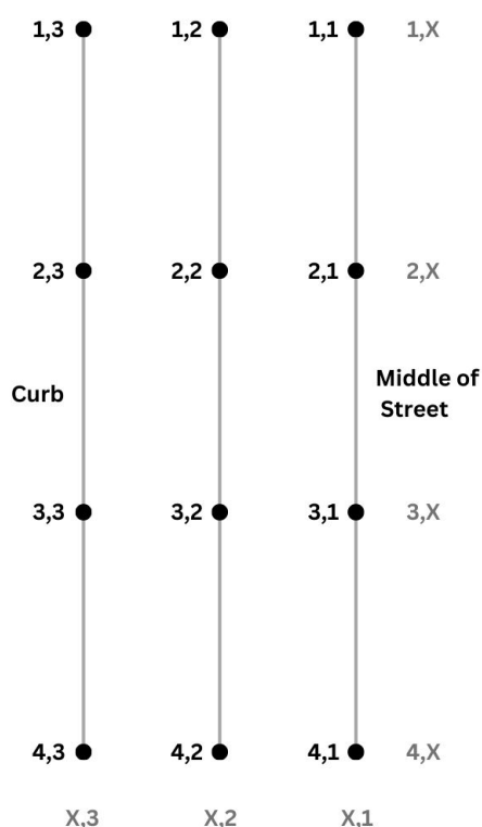
Figure 4. Diagram of the grid used to collect surface temperature measurements.
